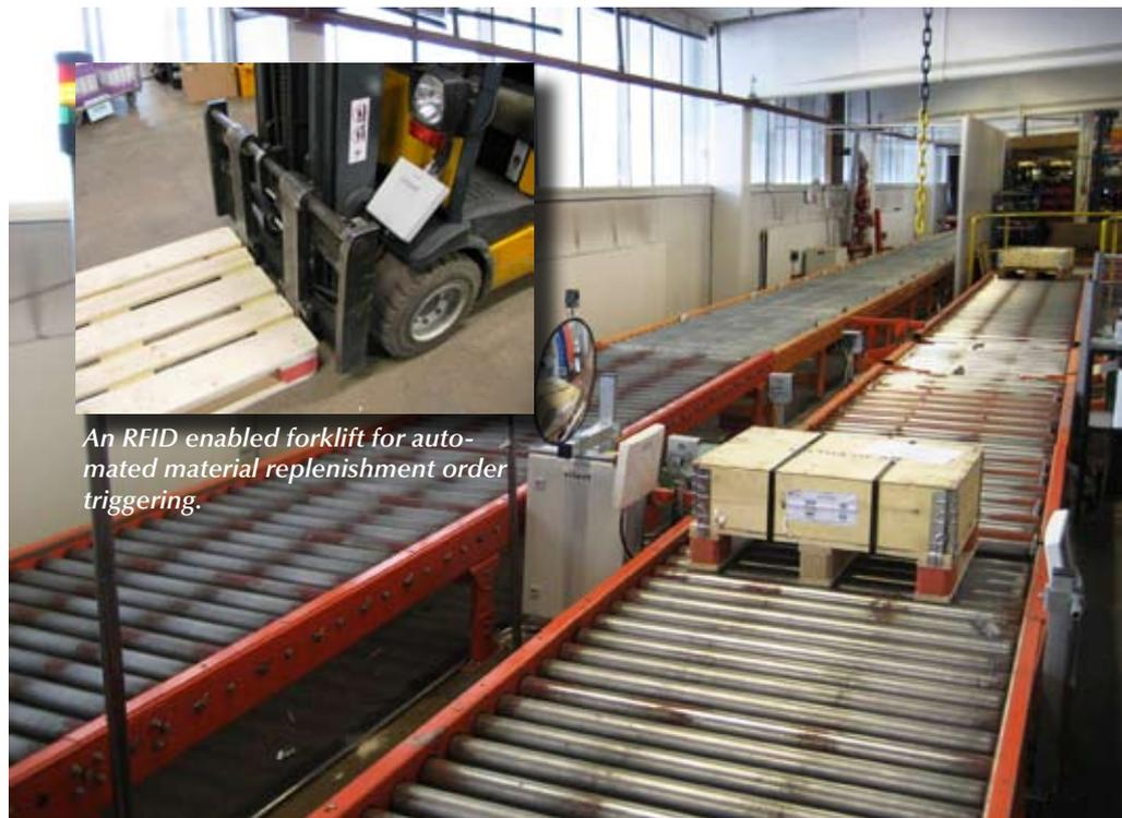
*An RFID enabled forklift for automated material replenishment order triggering.*
