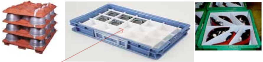
Returnable dunnage that protects and sorts parts
