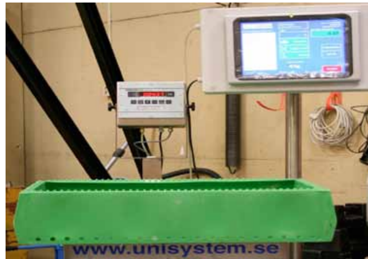
Weight scale with RFID and EPCIS report
