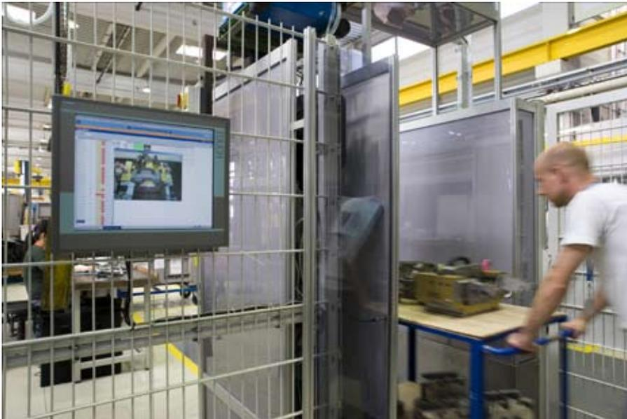
*Fig. 2: Expensive special tools (left) are managed with RFID at Siemens Power Generation. RFID antennas control the use of tools at the entrances to the production area (right).*
